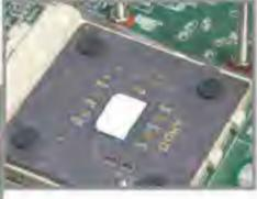
Note: Too much compound will decrease the performance of the CPU fan. The thickness should be between 1mm to 2mm.
